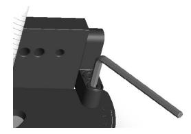
5. Use a precision square against the side of the miter bar without expansion discs to square the
