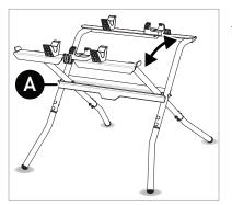
1. Open the stand, and then place on a solid level floor or solid level ground. The stand is fully opened when the center cross brackets (A) will not allow the stand to unfold any farther.
