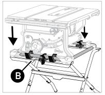
The cross plate with two cradles and one clamp is the front of the stand (B) (the rear cross plate has one cradle and one clamp). The front of the saw must face the front of the stand.
