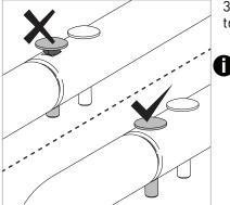
3. (cont.) Make sure the square shoulders of the bolts are inserted and mated to the square holes in the upper legs.
