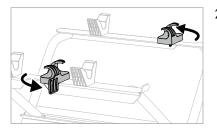
2. Open the clamps: pivot the front and rear clamps 90° counterclockwise.
