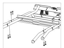
3. Insert the eight carriage bolts through the holes in the legs. You can insert the bolts from either side of the tubes.
