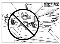
Always orient the front of the saw to the front of the stand. Do not attempt to mount the saw as reversed or turned sideways. This illustration shows the back of the saw towards the front of the stand.
