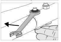
4. Thread the eight lock nuts onto the bolts, and then tighten all of the lock nuts except the adjustable right rear leg.
