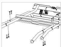
3. Insert the eight carriage bolts through the holes in the legs. You can insert the bolts from either side of the tubes.
