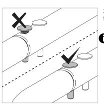
3. (cont.) Make sure the square shoulders of the bolts are inserted and mated to the square holes in the upper legs.
