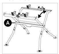
1. Open the stand, and then place on a solid level floor or solid level ground. The stand is fully opened when the center cross brackets (A) will not allow the stand to unfold any farther.
