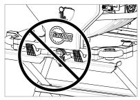
Always orient the front of the saw to the front of the stand. Do not attempt to mount the saw as reversed or turned sideways. This illustration shows the back of the saw towards the front of the stand.
