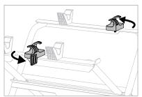
2. Open the clamps: pivot the front and rear clamps 90° counterclockwise.
