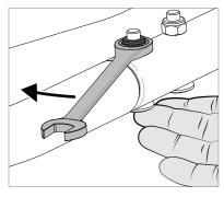
4. Thread the eight lock nuts onto the bolts, and then tighten. Do not over-tighten.
