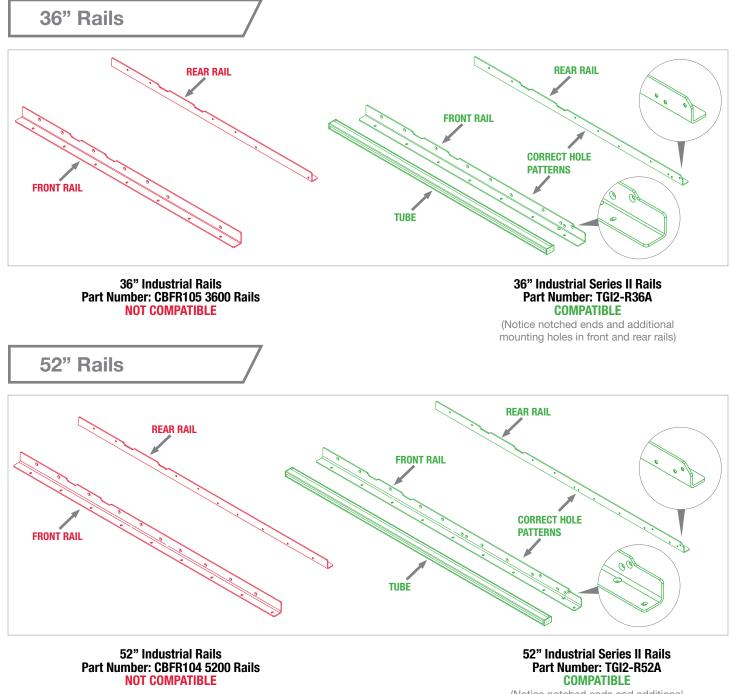
(Notice notched ends and additional mounting holes in front and rear rails)
