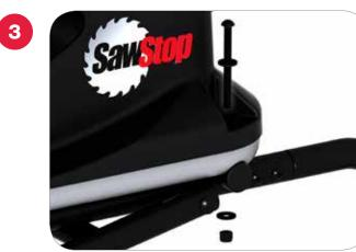
Remove each bolt along with the accompanied washers (2) and nut (1) from the cart and saw assembly using a 5mm allen wrench and a 13mm crescent wrench.
