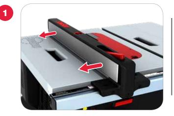
Slide the fence until the face of one side is flush with one of the miter gauge slots on either side of the table. If the fence is out of alignment, line up the fence and miter slot as close as possible to you.
