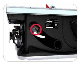
If a gap can be seen, locate the tilt angle rack adjustment screw on the inside of the cabinet. To access the screw for adjustment, go to the back of the saw and reach in through the dust collection port.
