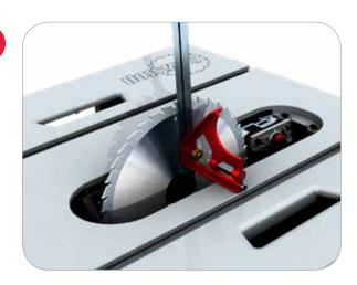
Using a combination square, place the flat edge of the square on the table so the ruler is parallel with the blade. Slide the combination square over until either the top or bottom of the ruler touches the blade.
