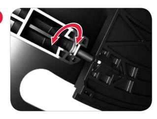
Using a 4mm ball end allen wrench, rotate the screw clockwise to move the top of the blade in towards the arbor arm and rotate counter-clockwise to move the top of the blade away from the arbor arm.
