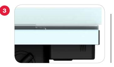
Once the straight-edge is correctly applied to the table top, evaluate the extension. If there is a gap between the extension and straight-edge, use a feeler gauge to determine how large the gap is. If the gap is no larger than .05in. the extension is aligned and requires no further adjusting. If the gap is greater than .05in, proceed to the remaining steps.
