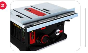
With the extension closest to the main table top, place a straight-edge across the top of the table from the motor side to the end of the extension. The straight-edge should be parallel to the rail.
