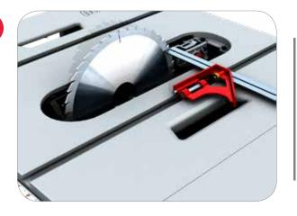
Slide the combination square along the miter slot towards the back of the blade (DO NOT LOOSEN THE RULER ON THE SQUARE). Rotate the blade towards the back of saw making sure to use the marked tooth to align with the ruler.
