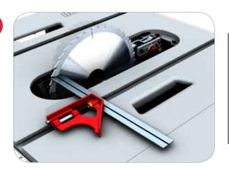
Using a combination square, set the edge of the square so it is parallel with the miter slot on the right side of the table. Extend the ruler out until it touches a tooth at the front of the blade. Mark that tooth with a felt top permanent marker.
