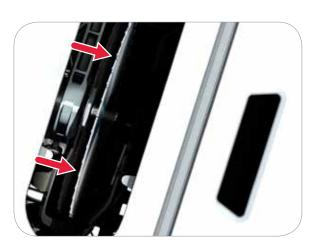
Loosen the arbor nut and slide the blade over to allow room for a 4mm allen wrench to be able to adjust the bolt. Rotate the bolt clockwise to move the blade right and counter-clockwise to move the blade left. Once adjusted, tighten the blade down.
