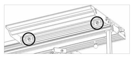
15. Slide the miter gauge bar (249) into the T-slot on the sliding table top <u>nearest</u> the blade, as shown in Fig. 11.
