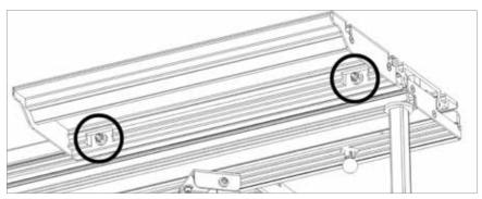
14. Slide the miter gauge bar (249) into the T-slot on the sliding table top <u>farthest</u> from the blade, as shown in **Fig.6**. For full cutting capacity, the miter gauge bar should be positioned flush with the front edge of the sliding table. Use a 5mm wrench to turn the **reverse-thread** fasteners (248) at the front and rear of the miter gauge bar <u>COUNTERCLOCKWISE</u> to lock the miter gauge bar in place.
