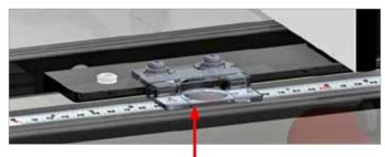
There should be a gap between the position indicator lens and the ruler on the main tube.
