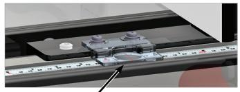
There should be a gap between the position indicator lens and the ruler on the main tube.
