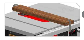
Lower blade to lowest elevation and turn off motor.
