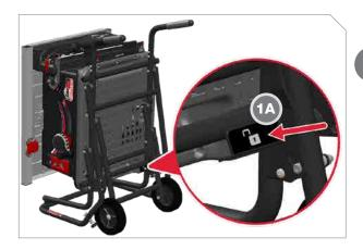
To open mobile cart, grasp both handles and raise cart and saw to upright position. Press lock release lever with right foot (1A) and pull handles toward you.
