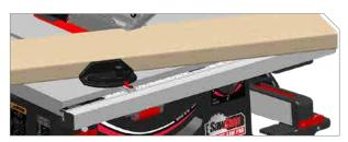
Make sure workpiece is not touching the blade. Turn on motor.
