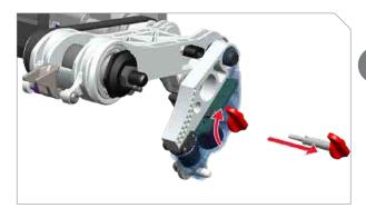
Turn brake key 1/4 turn clockwise and pull out.
