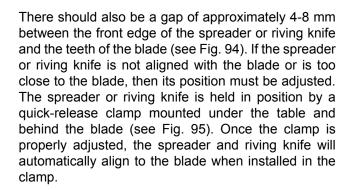
To adjust the clamp, set the tilt angle to  $0^{\circ}$  and remove the table insert. Remove the blade and set it aside. Make sure the spreader or riving knife is installed and lower the blade elevation to zero to provide access to the clamp.
