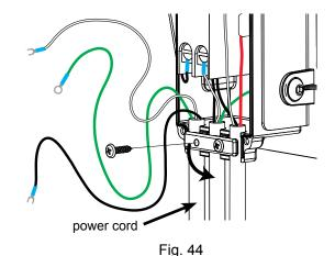
Now install the new power cord in the contactor box. Connect the ground wire (the green wire) to the ground, the white wire to the right, top terminal connection on the contactor, and the black wire to the left, top terminal connection on the contactor (see Fig. 45). A wiring diagram is shown in Fig. 46.
