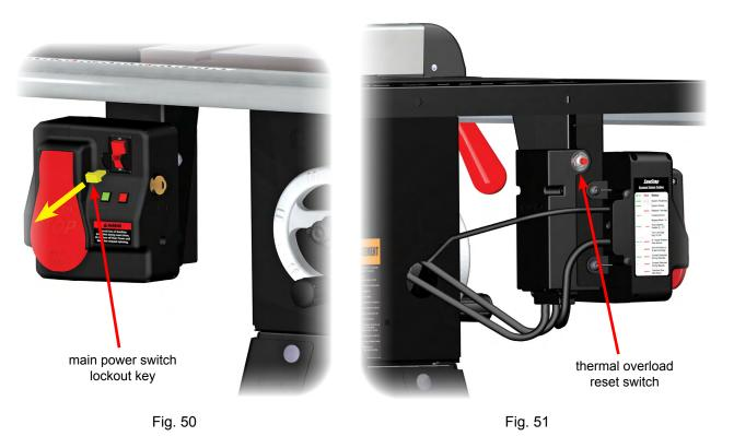
Your saw also comes equipped with a thermal overload switch that will cut power to the motor if the motor starts to overheat (see Fig. 51). The motor could overheat, for example, if it is overloaded or if a workpiece is fed too
