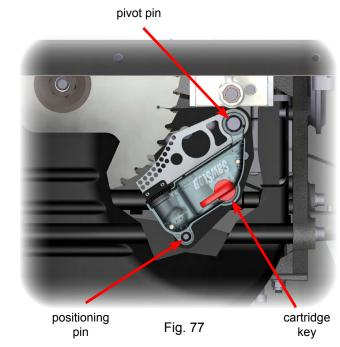
To remove the cartridge, first remove the cartridge key by turning it 90° clockwise and then pulling it away from the cartridge (see Fig. 78). Set the cartridge key aside for use with the new cartridge.
