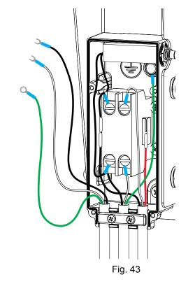
Using a Phillips screwdriver, remove the left screw that attaches the bar across the cords entering the contactor box and loosen the right screw. Then rotate the bar downwards far enough to remove the power cord (see Fig. 44).
