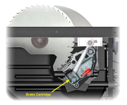
fiber materials, mirrored acrylic, carbon-filled materials, etc., will typically cause the brake to activate. If you need to cut these conductive materials, the safety system can be placed in "Bypass Mode" to temporarily disable the brake. (The Bypass Mode is discussed on page 55.)
