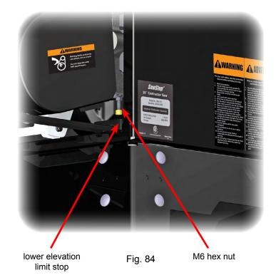
The purpose of the rubber bumper is to absorb the energy of the arbor block when the blade retracts below the table upon activation of the safety system. As shown in Fig. 85, the lower elevation limit stop should be adjusted so that the arbor block slightly compresses the bumper at the lowest elevation. This should also ensure that a 10 inch blade is at least  $\frac{1}{8}$  inch below the top of the table.
