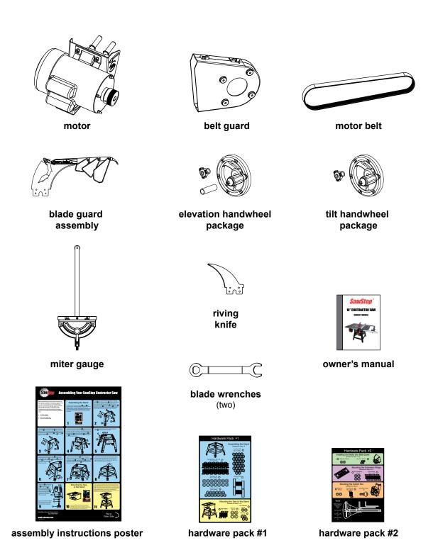
The instructions to assemble your saw are on a poster included with your saw and are listed below. You can follow either set of instructions to assemble your saw. In addition to the tools included with hardware pack #2 you will also need the following tools to complete the assembly: an 8 mm socket, a 10 mm wrench, two 13 mm wrenches, and a level or straight edge.
