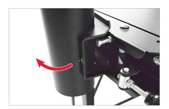
Loosen the Nut - M8 x 1.25 [T] using a 13mm wrench and thread the Bolt - M8 x 1.25, 45mm, Hex Head [V] in or out relative to the dust collection guard mounting bracket. Once the bolt is in the correct position, use a 13mm wrench to re-tighten the nut in order to secure the bolt.
