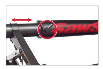
Tighten the inner dust tube lock knob by turning the handle clockwise. Do not over-tighten the inner dust tube lock knob.
