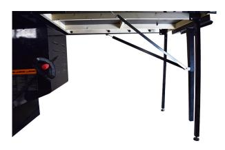
8 Check to make sure the **Extension**Leg [A] is still vertical and make any necessary adjustments.
