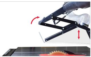
There are some operations in which the use of the floating dust collection guard system is not practical, and in those cases, the floating blade guard can be lifted up towards the dust tubes and the floating guard lock handle can be tightened to secure it in place.
