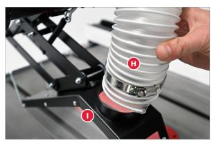
Using a screwdriver, tighten the included hose clamps to secure the dust hose both fittings described in steps 1 and 2.
