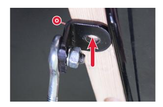
Pivot the leg support bracket back down to rest on the floor. Drill a pilot hole in the location you marked in step 3 with a 7/64" drill bit. Be sure to drill into the cross-support frame if you have a 36" extension table.
