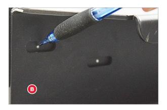
Locate an additional mark using the upper round hole where the Upper Leg [C] is joined to the Dust Collection Guard Mounting Bracket [B] to locate the mark.
