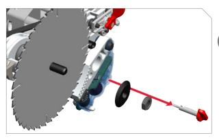
Remove table insert and riving knife or blade guard. Remove brake key, arbor nut, and washer.
