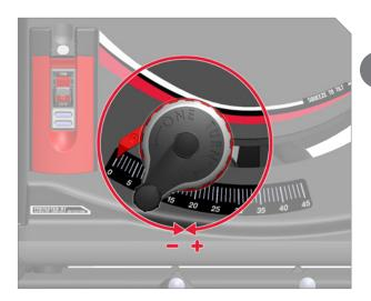
Switch power off and unplug the power cord. Rotate elevation handwheel fully counter-clockwise then fully clockwise to reset blade.
