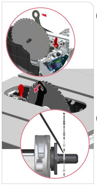
Use blade wrench to push brake slightly toward end of mounting pins.
