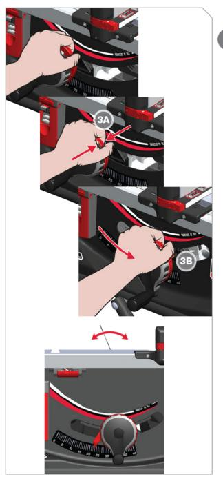
Change tilt angle by squeezing backplate against hand wheel (3A) and sliding hand wheel to side (3B) . Release backplate to lock blade in place. This adjusts tilt angle in single degree increments.
