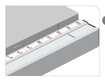
Use a pencil to mark the extension table and rail in the same location for alignment purposes in later steps, or make note of where end of table meets rail ruler.
