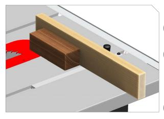
Adjust blade elevation to the desired grooving depth.
