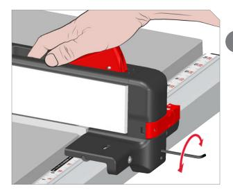
Unlock fence and insert a 3 mm hex key wrench into hole in front of fence. Turn clockwise to tighten or counter-clockwise to loosen. Check clamping force by locking and unlocking fence several times. Make further adjustments as necessary.
