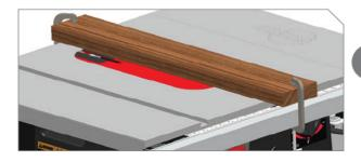
Clamp a thick piece of wood across right side of table insert to securely hold table insert to table.
