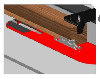
Use a push block or push stick to safely cut workpiece. Turn off motor.
