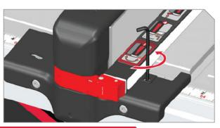
Use a 3 mm hex key wrench to loosen bolt next to indicator lens.
