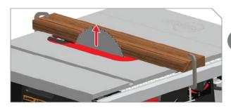
Start motor and slowly raise blade (see page 38) to its highest elevation. This will create the slot for cuts at zero degrees tilt.
