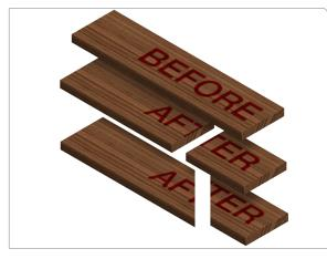
Cross-cutting (cutting perpendicular to the grain of the workpiece) is performed using a miter gauge. The miter angle is indicated by the scale below the pointer.
