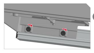
Once table top and extension table top are aligned, and the marks are aligned, open extension table and tighten screws.
