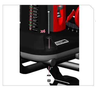
Use 5 mm hex key wrench and 13 mm wrench to remove hardware from saw corners.
