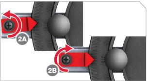
Check that the angle marker is set at 90 degrees. If adjustment is needed, use a Phillips head screwdriver to loosen screw (2A), adjust angle marker to 90 degrees (2B), and re-tighten screw.
