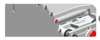
Remove table insert and blade guard. Raise blade.
