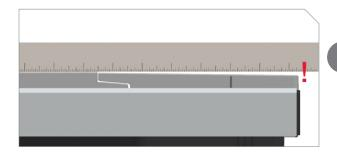
Check for gap between extension table and straightedge. If there is a gap, use a feeler gauge to determine size. If gap less than 0.05" (1.3 mm), extension table aligned, so no adjustment needed. If gap is larger than 0.05" (1.3 mm), proceed to next step.
