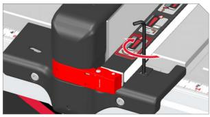
Tighten bolt. Check position of lens and make further adjustment as necessary.
