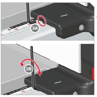
Insert 3 mm hex key wrench (3A) at an angle into hole in left side of fence head. Rotate screw (3B) clockwise to shift fence left, or counter-clockwise to shift fence right. Lock fence and check alignment. Make further adjustments as necessary. When fence is parallel to the miter slot, tighten screw in top left side of fence head. (Reverse Step 2)
