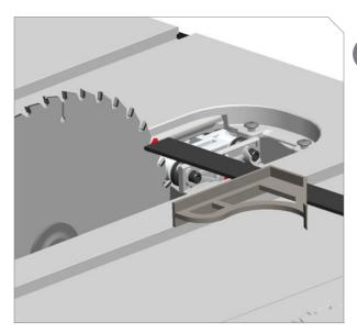
Set combination square parallel with right miter slot. Extend ruler until it lightly touches the side of the marked tooth. Tighten the locking knob on the combination square.
