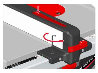
Unlock fence. Use a 3 mm hex key wrench to slightly loosen screw in top left side of fence head.
