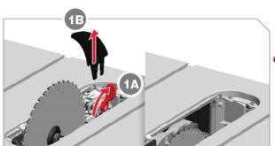
The blade slot in original insert is pre-cut at factory. However, you must cut a slot in any replacement inserts.
