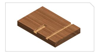
Dado cuts are used to create a slot or trench in the surface of the workpiece. A Dado is cut perpendicular to the grain of the workpiece.
