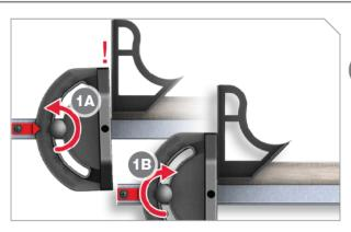
Loosen handle (1A). Use a combination square to ensure that bar and gauge are perpendicular. Tighten handle to lock head (1B). Recheck alignment and make further adjustment as necessary.
