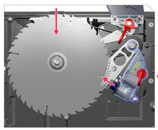
Upon brake activation, blade will stop spinning and may drop below table (unless blade was spinning slowly). You must change brake and blade to reset your saw.
