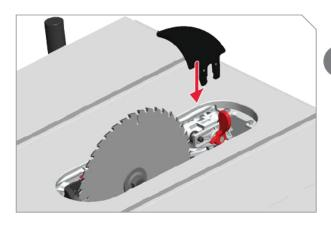
A primary reason to use the riving knife is for non-through cuts where the blade guard and splitter cannot be used.
