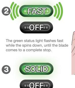
When the green light is solid, the saw is ready to shut off.
