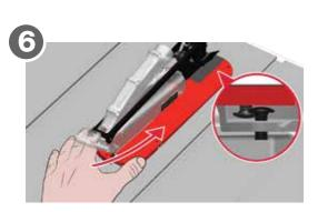
With the rear of the table insert tilting downward, slide the table insert into the table opening so that the screws on the bottom of the table insert slide beneath the screws in the table.
