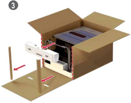
Cut both vertical edges of the box on the end near the wheels and fold down. Remove the small packing tray by sliding out from the cart and set aside.
