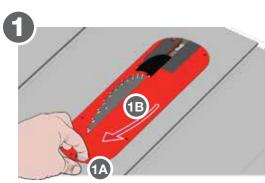
Squeeze the latch on the table insert (1A), and then lift the insert up and toward the front of the saw (1B).
