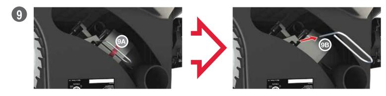
At the back of the saw, reach into the opening and remove a piece of red tape that holds a metal shipping pin in place (9A). Then pull the metal shipping pin completely out of the saw (9B). This pin holds the elevation mechanism in place during shipping and can now be discarded.
