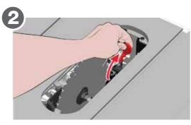
Open the clamp by reaching into the opening and flipping the red handle up.
