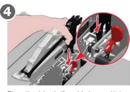
Place the riving knife or blade guard into the clamp.
