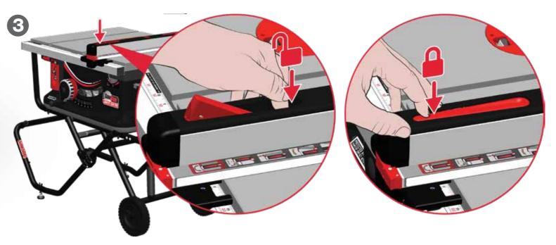
Align the fence on the front rail and slide it to the desired cutting position. Press the red lever to lock the fence in place.
