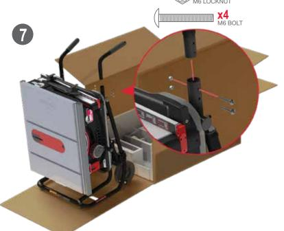
Slide the handle marked "L" into the tube nearest the front of the saw and bolt in place. Tighten the bolt enough to compress the tubes so the handle does not jiggle. Install the handle marked "R" in the same way in the other tube.
