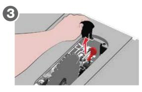
Slide the riving knife or blade guard out of the clamp.
