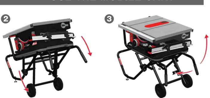
Pull the handles downward. The wheels will swing down and to the rear. The cart will lock in place once the saw is in the full upright position.
