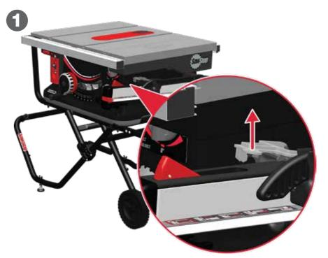
The rip fence is stored in brackets on the right side of the saw, beneath the table extension. Lift the gray latch to remove the fence.
