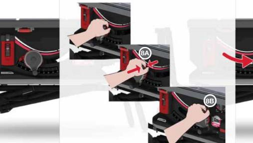
Do not attempt to elevate the blade until steps 8 and 9 are complete. Roll the saw off the cardboard. Tip the saw down to rest on the cart handles. Grasp and squeeze the backplate against the elevation handwheel (8A) and swing the handwheel to the right (8B) until the red pointer is over the 45 degree mark (8C). Release the backplate to lock the tilt at 45 degrees.
