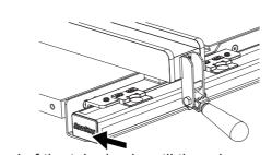
Push the left end of the tube back until there is approximately a 1/32" gap between the rail and glide plate. You can insert one credit card or two business cards between the rail and guide plate to gauge the distance. Remove the fence and turn the parallelism screws, as needed-turn the screws in very small increments.
