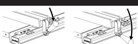
Lock the fence, and then follow the next steps to check the gap between fence and the front rail. Turn the parallelism adjustment screws clockwise to reduce the gap, counterclockwise to increase the gap. The parallelism screws also adjust clamping pressure-the
